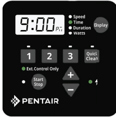
Figure 7: Activating External Control Only
