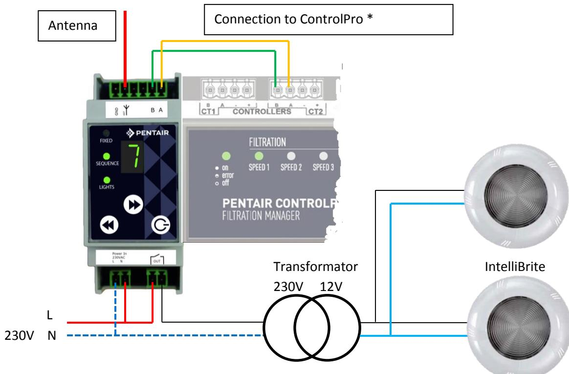
In most cases the antenna supplied with the system is sufficient. It is however possible to connect an external antenna to increase performance of the remote control. In such case connect the core of the cable to ANT and the metallic shielding to GND.
