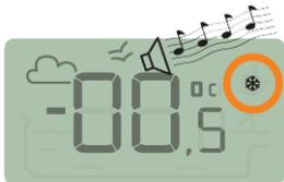
The gel pictogram related to the air temperature is displayed if the temperature measured by the Radio Relay is less than +3°C.
