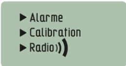
The Alarm (Alarm mode [→Page 65]) and Calibration modes (Calibration mode [→Page 67]) correspond to the position of the switch on the back of the Inner Display.
