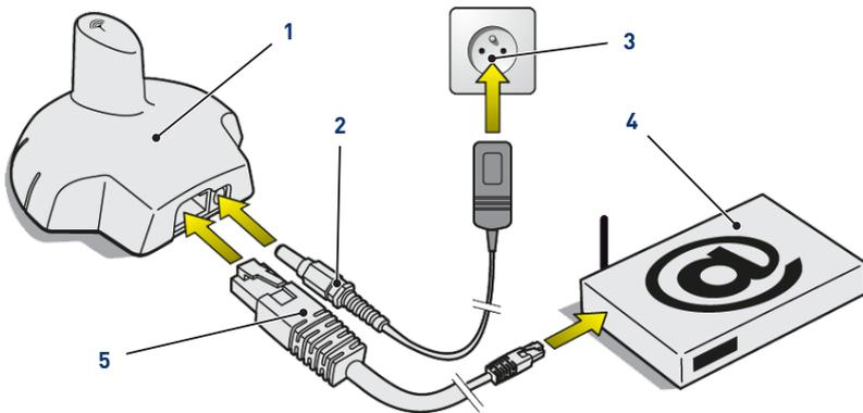
1. Connect the provided Ethernet cable (5) to the Internet Relay (1) and your internet modem (4).
