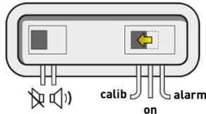
⇒ Calibration mode is selected on the Inner Display:
