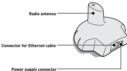
This relay, once connected to your internet box (see Internet Relay [->Page 27]), created a radio network allowing it to send and receive information from your installation.
