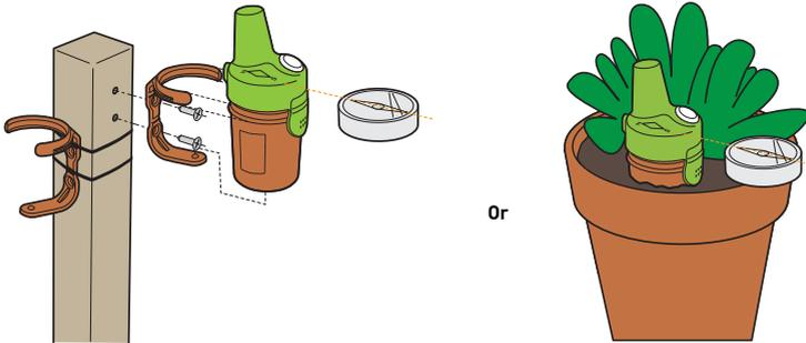
2. Place the Radio Relay according to one of these configurations:
