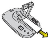
2. Remove the insulating film from the batteries.
