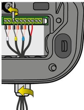
1. Unscrew the cable gland completely: be careful not to drop the black flexible seal.
