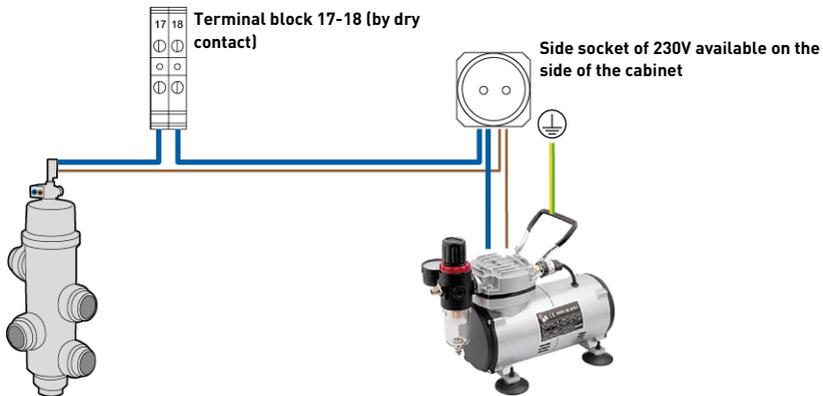
**Connection of an electric heater**
