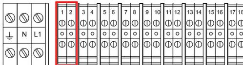
In case an electrolyser of another brand is used, you can use the control of dry contacts by means of terminals 13 and 14.
