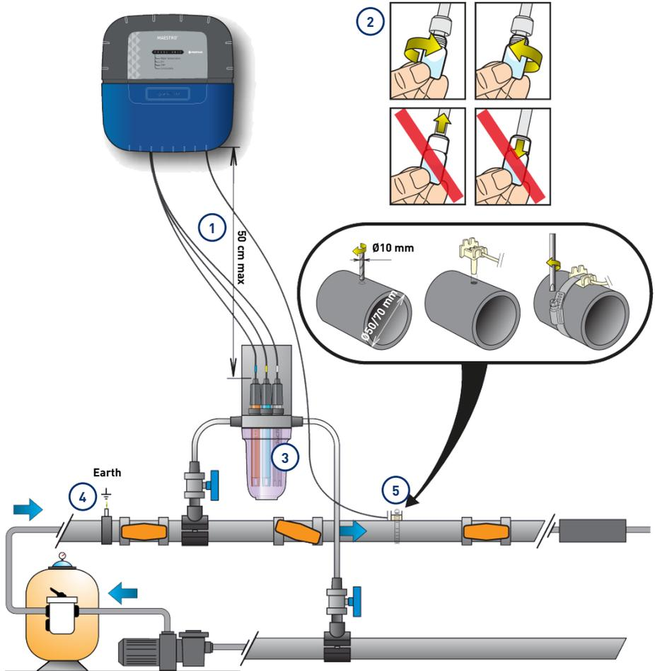
**1** The probe cables must not cross the power cable (risk of interference) or be wound on themselves.
