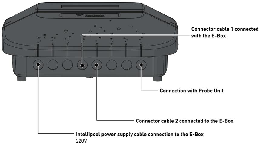
Connections to be made to the Control Centre box, through the fast cables (provided).
