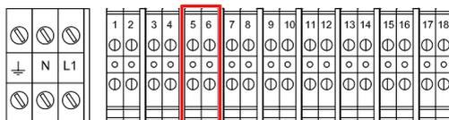
The connection of the control cable must be carried out on the Bus + and – terminal blocks of the INTELLIPOOL (Control Centre or Probe Unit).
