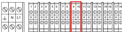
**4.8.8 Connection of the chlorine pump power supply**
