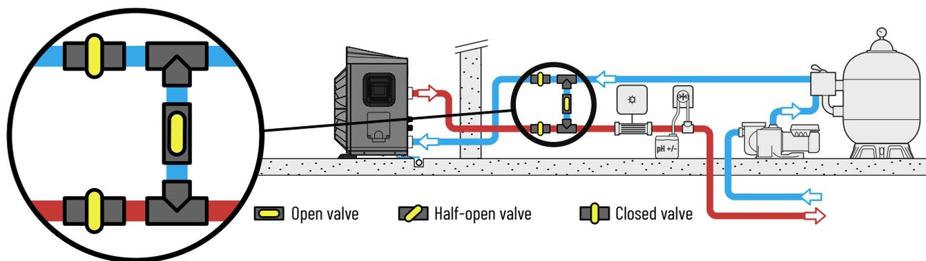
3 - Unscrew the junctions to evacuate all the water contained in the HP.
