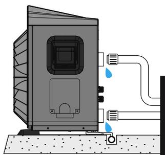
4 - Reconnect and slightly tighten the junctions by hand to prevent the introduction of foreign objects into the HP
