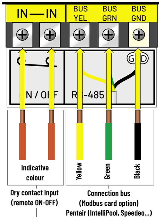
Dry contact input (remote ON-OFF), remove the shunt that is present
