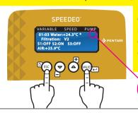
parameters while being fully aware of the consequences. In order to limit accidental access, the *Install menu* menu has secured access, (from the main menu, simultaneously hold down **Esc** and **Valid** for 3 secs. A star appears in the top right corner of the home screen).
