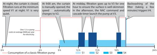
Consumption is roughly speed squared, so when the rotation regime is divided by 2, the electricity consumption of a pump is divided by 4! The average profit of SPEEDEO running a VS pump alongside a classic filtration of 1.5 cv is €450 per year (ERDF base rate in 2015).
