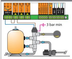
An outlet is a dry contact and does not supply any voltage.
